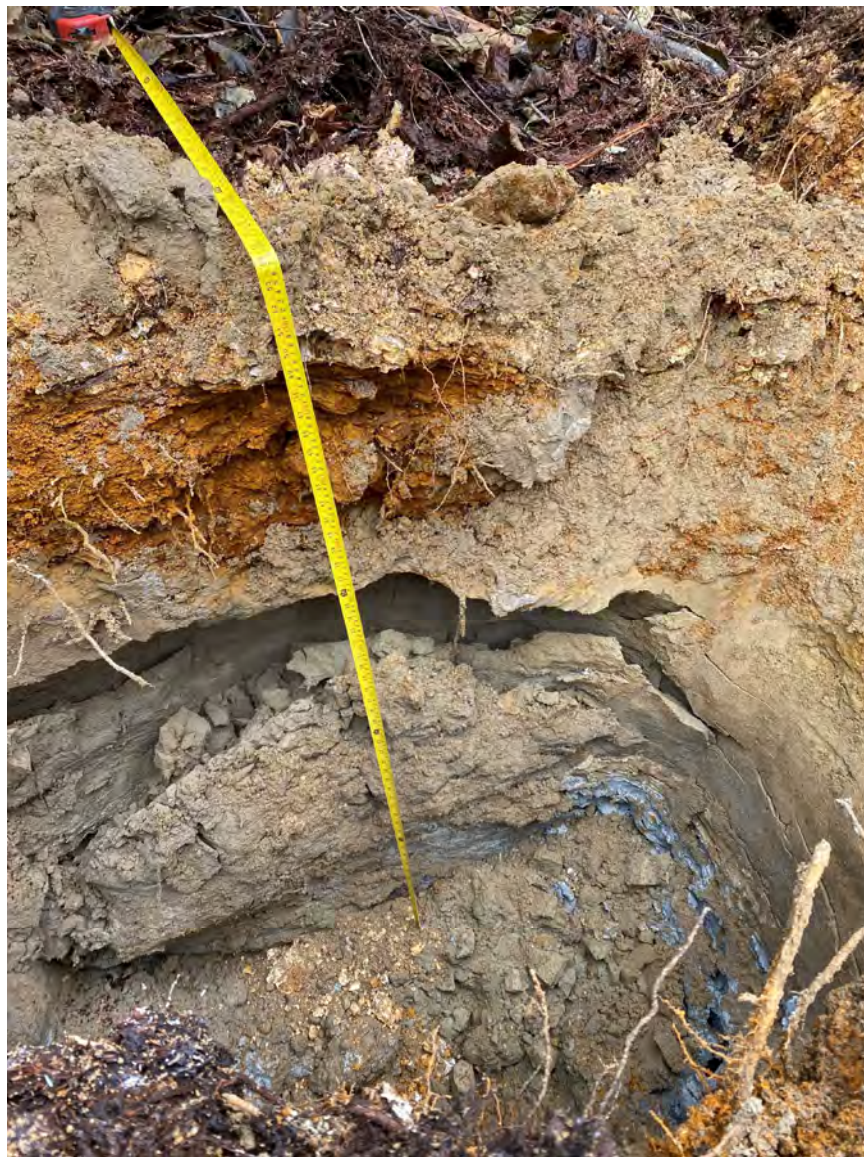
Figure 4: Example of typical tailings profile in test pit A06
