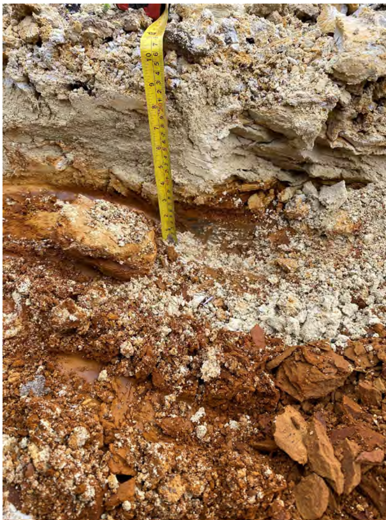
Figure 5: Hard ferruginous looking layer in test pit A04
