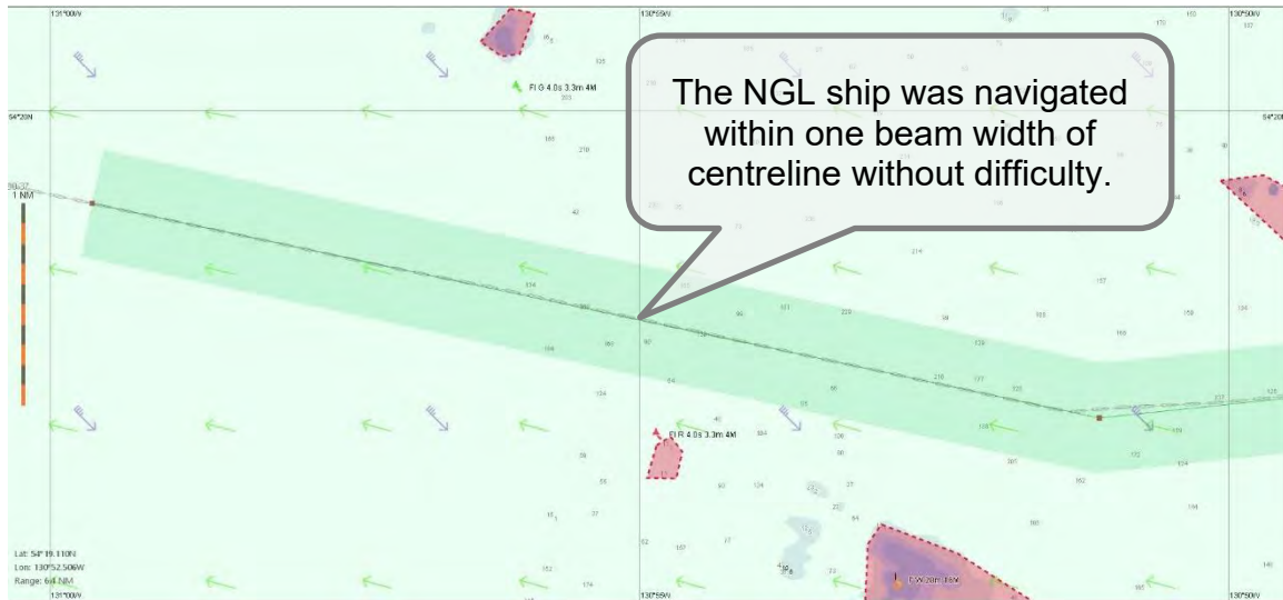
Figure 59: Track-plot – Pilot Station to Hanmer Rocks, wind NW 40 (R1-7)
