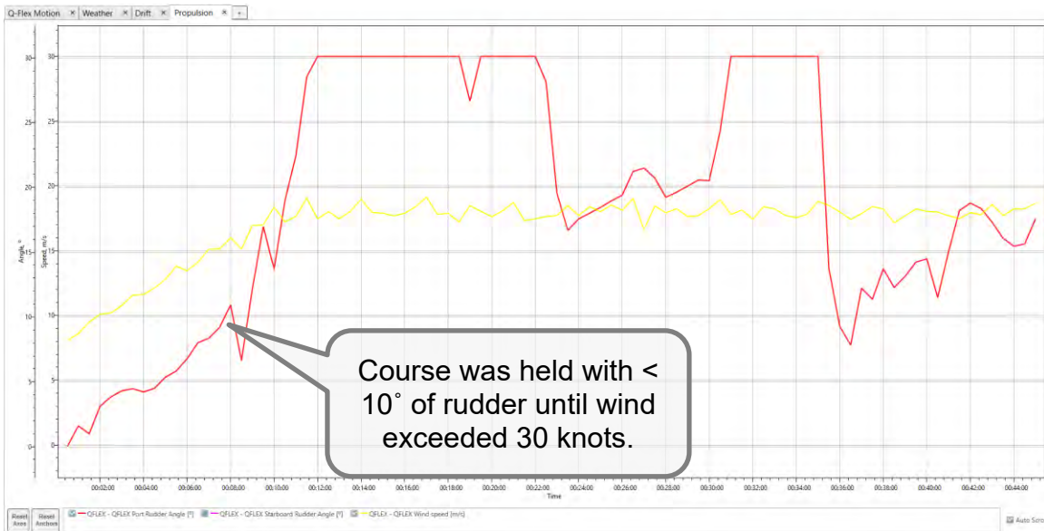
Figure 33: Wind vs rudder – Beaver Rocks to Triple Island, wind SE 35 (R1-2)
