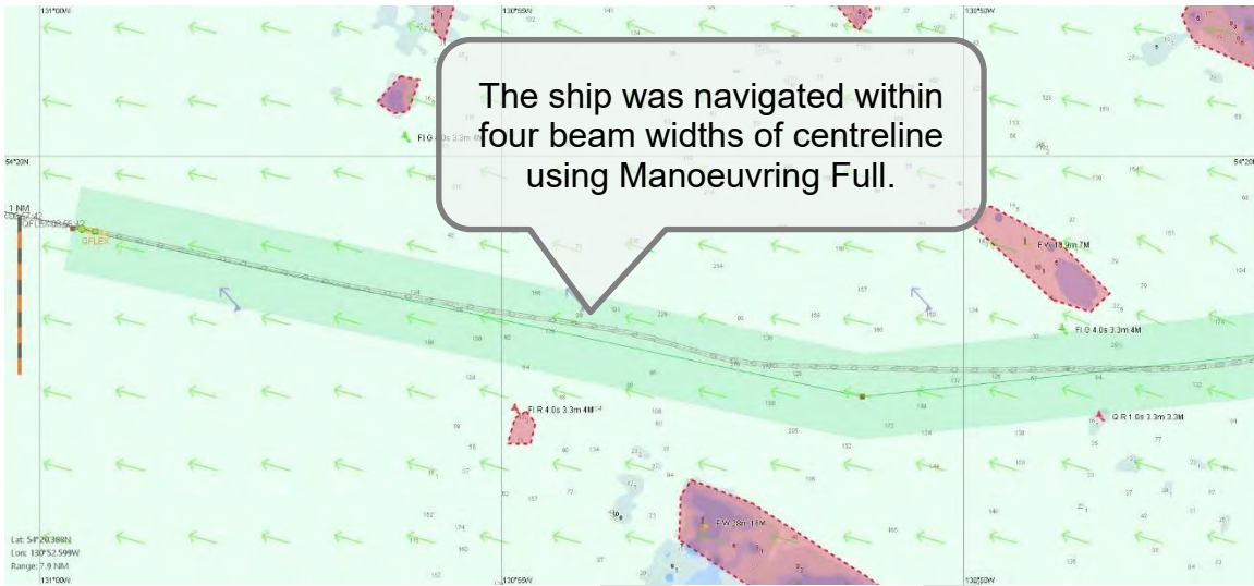
Figure 55: Track-plot – Hanmer Rocks to Pilot Station, wind SE 50 (R1-6)
