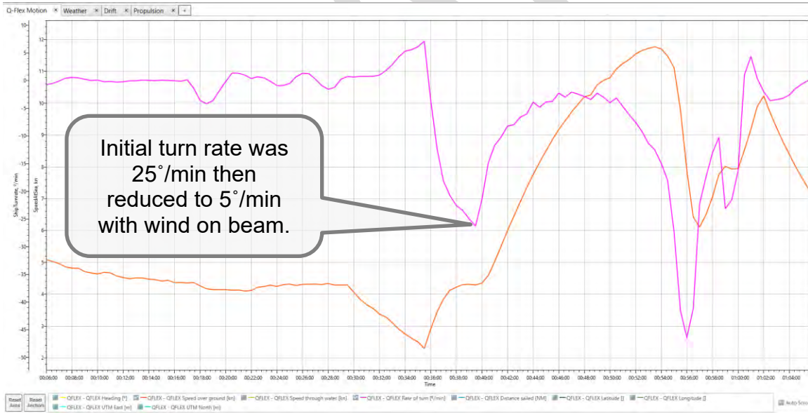
Figure 73: Rate of turn – turning stern through 50 knot winds (R1-10)
