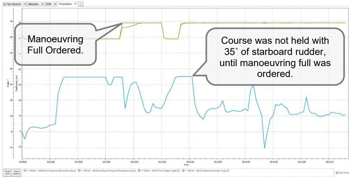
Figure 57: Applied rudder – outbound LNGC, wind SE 50 (R1-6)
