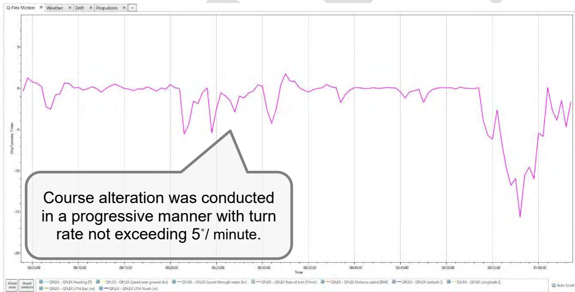
Figure 40: Rate of turn – inbound LNGC. Wind NW 40 (R1-3)
