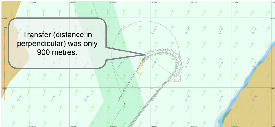
Figure 92: Tug assisted track-plot – high speed turn, 50 knot winds (R1-13)
