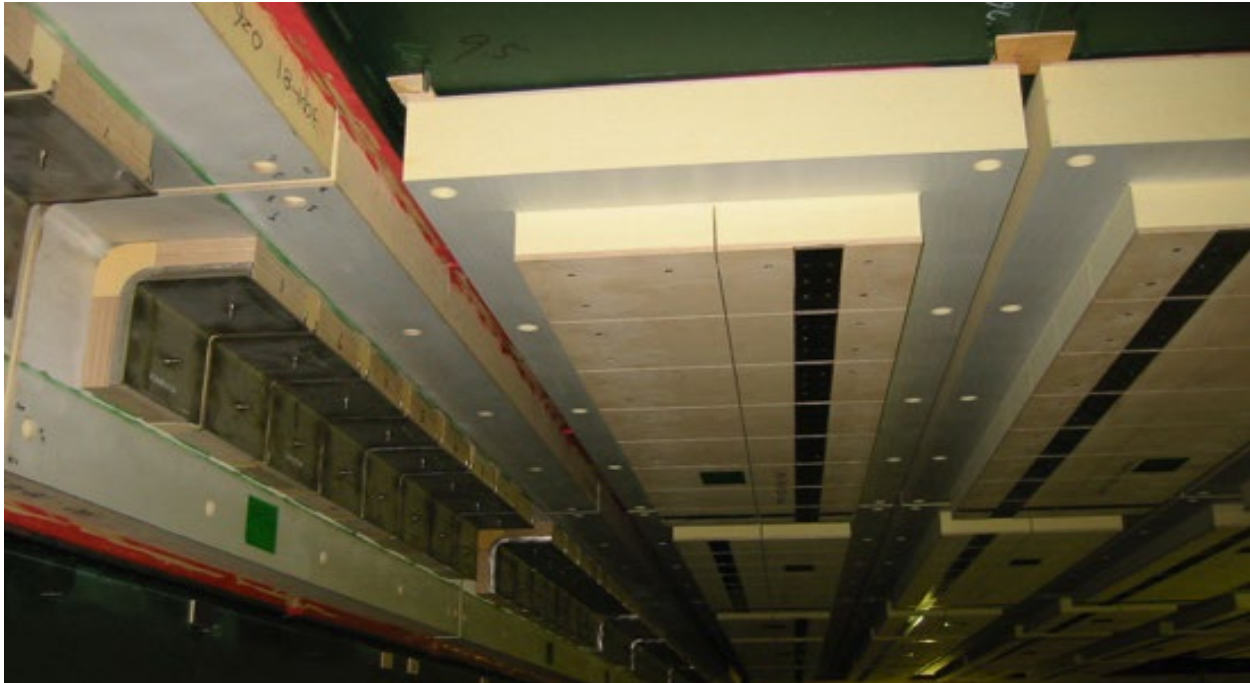
Figure 6 – GTT No. 96 Invar primary and secondary barrier
