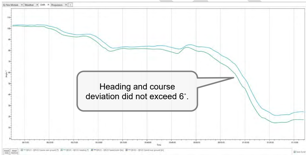
Figure 50: Drift angle – inbound LNGC, wind NW 50 (R1-5)
