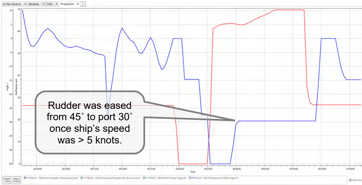
Figure 74: Rudder and RPM – turning stern through 50 knot winds (R1-10)
