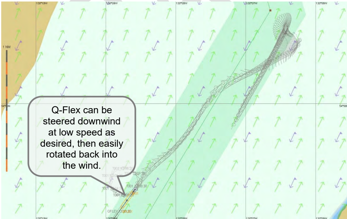
Figure 86: Tug assisted track-plot – falling off 50 knot winds (R1-12)
