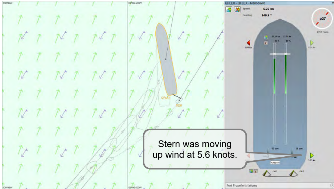
Figure 88: Tug assisted track-plot – initiating high speed turn, 50 knot winds (R1-13)
