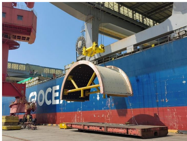
Ball mill shell segment in transit
