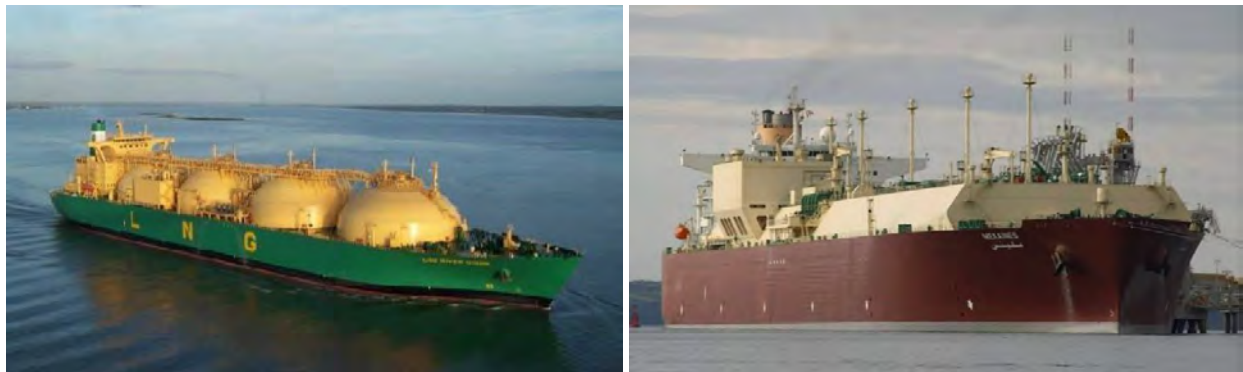
Figure 4 – Spherical-type LNG carrier (left) and membrane-type LNG carrier (right)
