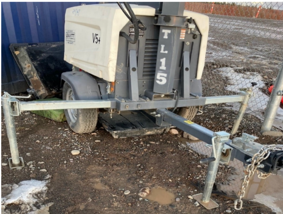
Photo 15: 7-Mile MUS light plant secondary containment re-positioned and dry.
