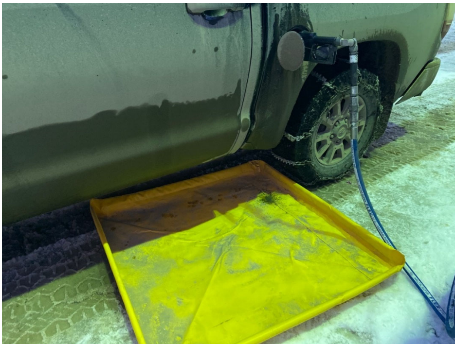
Photo 18: Drip trays in use while re-fueling at MUS 9A.
