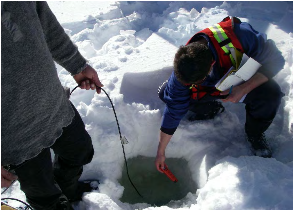
Photo 4: Obtaining pH and confirming temperature at Site 1.
