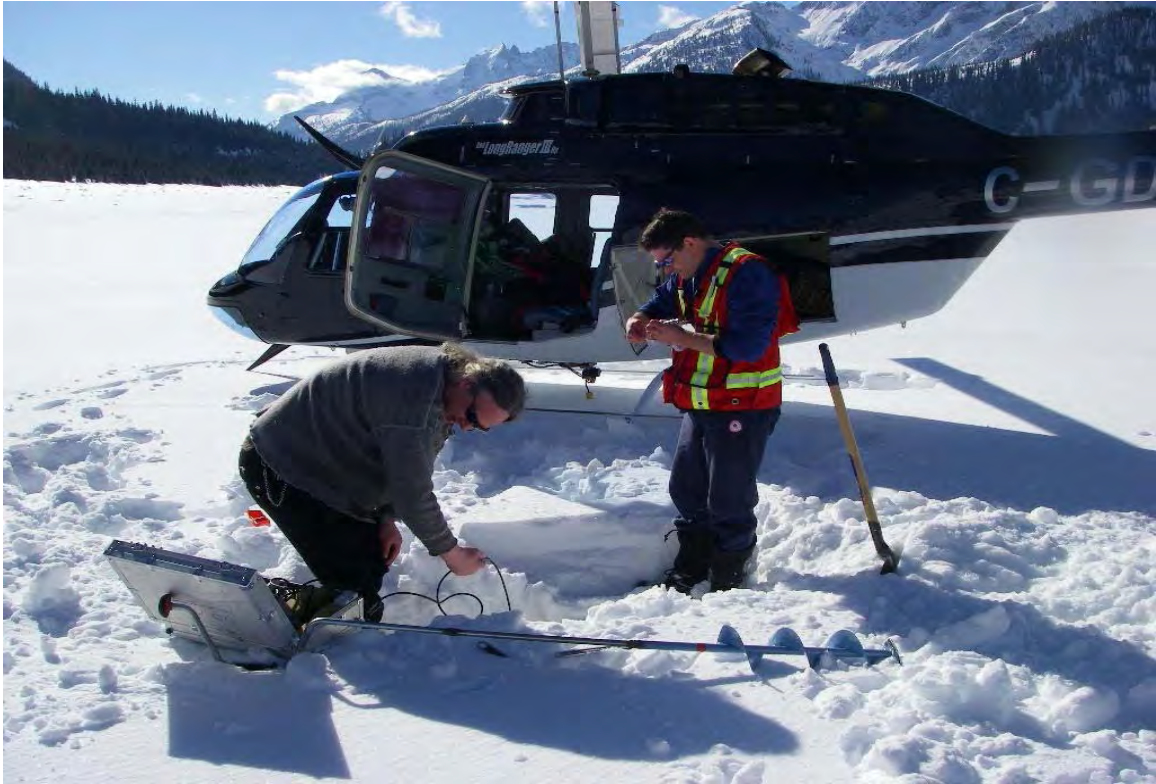
Photo 3: Obtaining the dissolved oxygen/temperature profile at Site 1 – the Northern Site.
