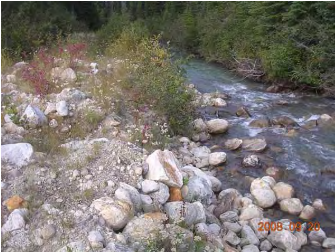
Photo 3: Stabilized left bank scour previously recorded at riffle #5 of the outlet channel.
