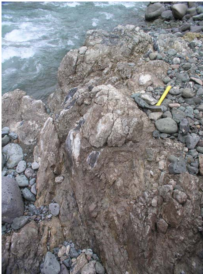
Photo 8. Shear zone contains limestone fragments in gouge - valley bottom NovaGold Mapping: P-Dam-6-60; Photo Date: 11 October 2005
