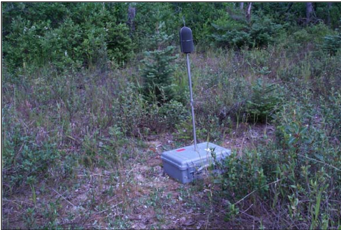
Plate 1-3 The Quest 2900 sound level meter with its environmental enclosure kit monitoring baseline noise levels during July 2005. The microphone is protected by a wind screen/weather shield and bird spikes. The weather resistant case protects the meter and battery pack and provides a stable base for the kit.
