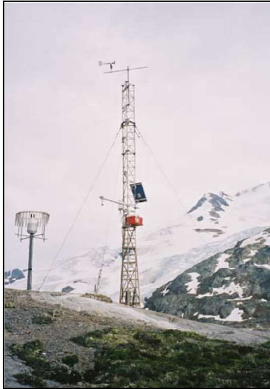
Plate 1-1 Meteorological station installed near West More Creek. The GEONOR precipitation gauge can be seen on the left.
