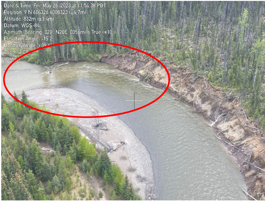
Photo 9. Eroding bank depositing sediment into Gosnell Creek downstream of the Project ROW.
