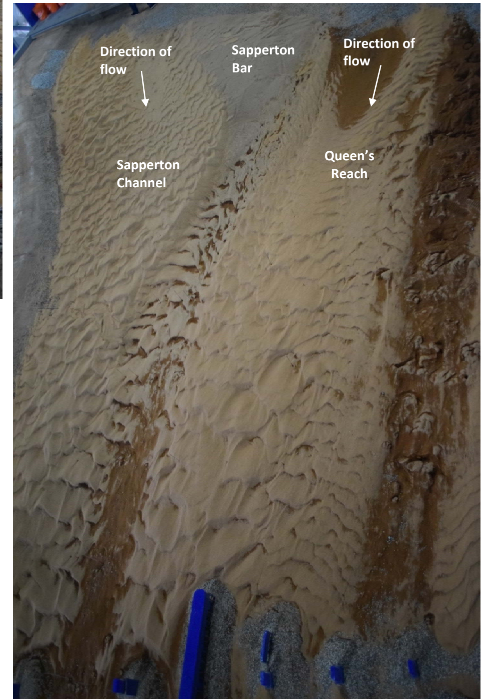
4) Overhead view of upstream reach of the physical model after the Baseline test at Flood of Record. (DSC 1009)
