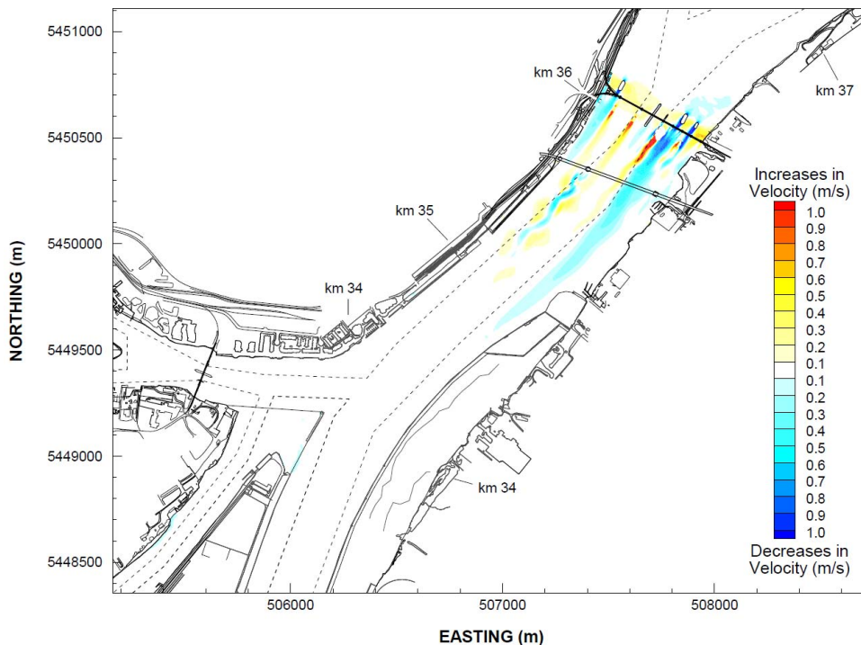
Figure 18. Difference in depth-average speed distribution – Decommissioning minus Existing Conditions
