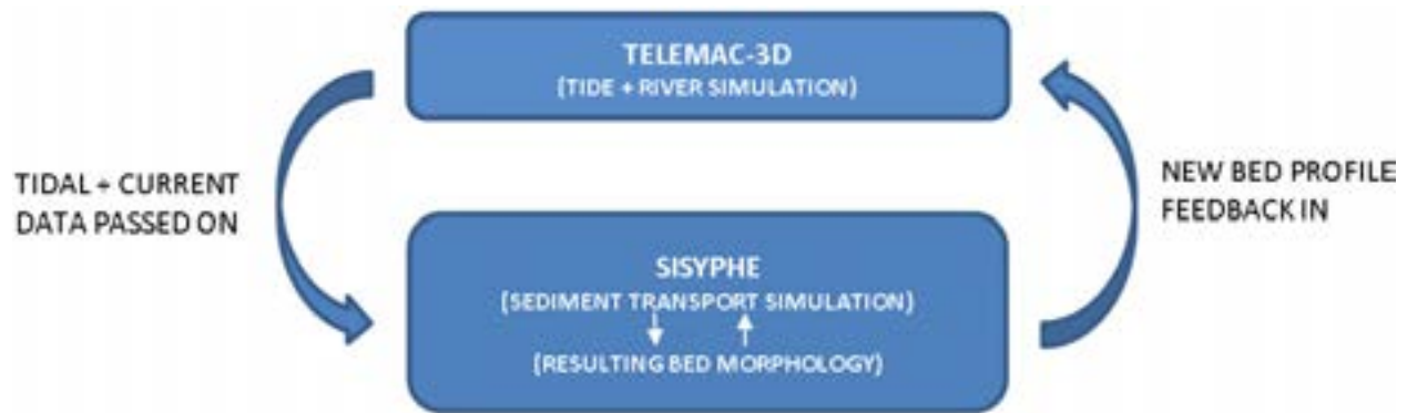
Figure 4.1-7 TELEMAC Model Coupling Flow Diagram
