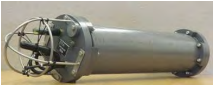
Figure 1. Autonomous Multichannel Acoustic Recorder (AMAR; JASCO Applied Sciences).
